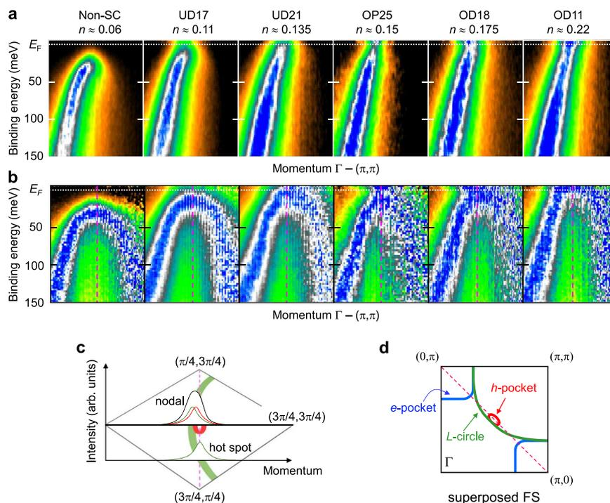
**Fig. 2 | Doping evolution of the nodal band in PLCCO.** **a** ARPES spectra of the nodal band after Fermi–Dirac correction for various doping samples. OP indicates optimal doping. **b** Nodal band spectra with the maximum energy distribution curve (EDC) that brightens the “folded shadow band” forbidden in **(a)** (see Supplementary Fig. 3). **c** Schematic spectra of the FS at the nodal point and hot spot. The black
