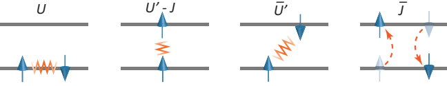
FIG. 3. On-site interactions within one quantum dot: Hubbard U , interorbital Hubbard U' (and its spin-antiparallel form \bar{U}' ), and Hund's exchange J (and its spin-antiparallel form \bar{J} ).
